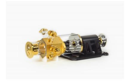
Fig. 2: The Radiometric Calibration Spectral Source (RCSS) realized at Fraunhofer IOF was used to calibrate one of the Webb measuring instruments on the ground. © Fraunhofer IOF
